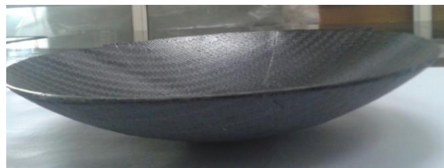
Fig. 3. Composite cured antenna reflector
