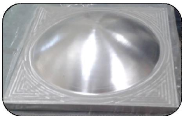
Fig. 1. The paraboloid stainless steel mould
